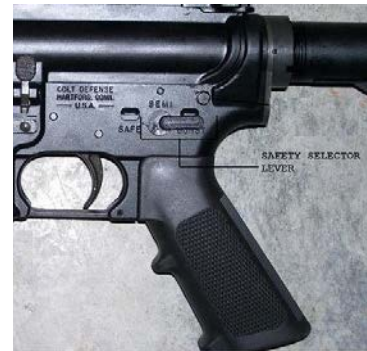
Figure 6. Selector Switch on Safe
