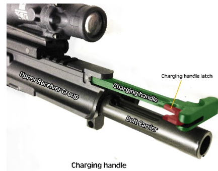
Figure 8. Removing the bolt carrier
